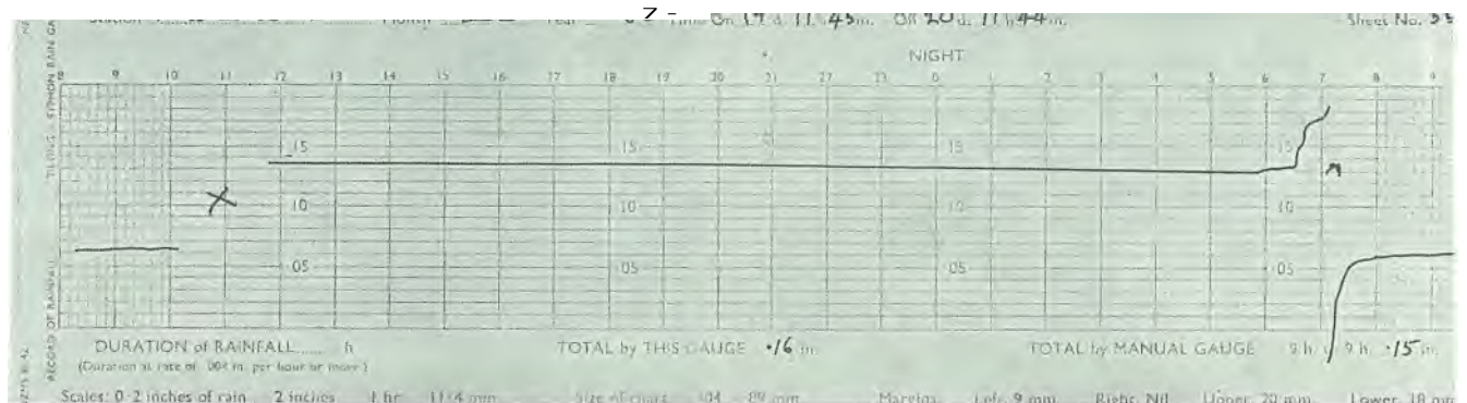
Fig. 3: A sample daily tilting syphon rain gauge chart.
